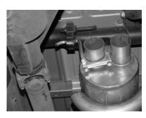
INSTALL MUFFLER #B ONTO HEADPIPE AT LEAST 1 ½" TO 2". USE CLAMP #F TO SECURE MUFFLER TO HEADPIPE. DO NOT TIGHTEN. USE A JACK STAND TO SUPPORT THE MUFFLER. OUTLETS SHOULD BE AT THE TOP.
