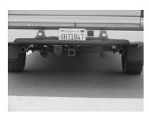
INSTALL EXIT PIPES #E ONTO TAILPIPES. CUT TO YOUR PREFERED LENGTH USE CLAMPS #G TO SECURE EXIT PIPES TO TAILPIPES. THESE CLAMPS ALSO ATTACH TO METAL HANGERS #H. THESE METAL HANGERS NEED TO BE ROTATED IN ORDER TO ADJUST FOR CLAMPING. NOW YOU CAN TIGHTEN ALL CLAMPS, NUTS, AND BOLTS, STARTING FROM THE FRONT WORKING BACK. USE ZIP TIES TO TIE AWAY BRAKE LINES. IF YOU WOULD LIKE YOUR EXIT PIPES TO EXIT BEHIND THE REAR WHEELS ROTATE THEM TO DO SO. INSTALL STAINLESS TIPS.
