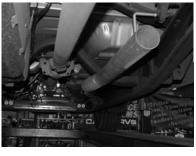
INSTALL PASSENGER SIDE TAILPIPE #C INTO MUFFLER AT LEAST 1 ½" TO 2". USE CLAMP #G TO SECURE PIPE TO MUFFLER. DO NOT TIGHTEN. THE TAILPIPES WILL BOTH LEAN TOWARDS THE DRIVER SIDE FOR CLEARANCE.
