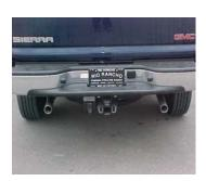
Install driverside overaxle tailpipe #E into muffler  $1 \frac{1}{2}$ " to 2". Use clamp #I to secure pipe to muffler. Do not tighten. Next, insert welded hanger into rubber grommet. Rotate pipe until it connects with rear hanger. Attach clamp #I to tail pipe.
