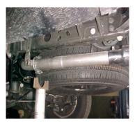
USE CLAMP # I TO SECURE TO THE MUFFLER, INSERT WELDED HANGER INTO THE RUBBER GROMMET. DO NOT TIGHTEN. NEXT, INSTALL THE EXIT PIPES # E AND #F. USE CLAMPS # H TO SECURE TO THE TAILPIPES. DO NOT TIGHTEN. USE ZIP TIES TO SECURE BRAKE AND FUEL LINES AWAY FROM
