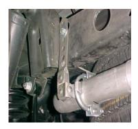
INSTALL METAL HANGER # I INTO HOLE LOCATED APPROXIMATELY 23" FROM THE REAR OF THE FRAME. USE TOP HOLE ON HANGER. INSTALL DRIVER SIDE OVERAXLE TAILPIPE # C INTO THE MUFFLER 1-1/2"-2". USE CLAMP #H TO SECURE PIPE TO MUFFLER.DO NOT TICHTEN
