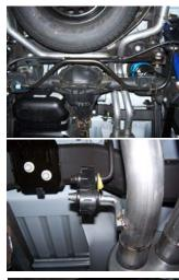
**7.** Install driver side tailpipe #C to the muffler 11/2-2". Use clamp #H to secure tailpipe to muffler. DO NOT TIGHTEN. Insert welded hangers into rubber grommets.
