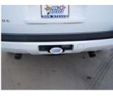
9. Install stainless steel tips. Clamp down. When you have everything in place, firmly tighten all bolts and clamps down securely. Use stainless steel cleaner and a Scotch Brite pad weekly to prevent tip from discoloration. Inspect all fasteners after 25-50
