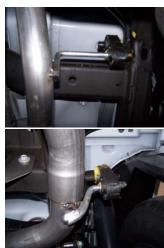
5. Install passenger side tailpipe #D to the muffler 11/2-2". Use clamp #H to secure tailpipe to muffler. DO NOT TIGHTEN. Insert welded hangers into rubber grommets.
