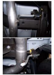
**5.** Install passenger side tailpipe #D to the muffler 1½-2". Use clamp #G to secure tailpipe to muffler. DO NOT TIGHTEN. Insert welded hangers into rubber grommet.
