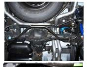
7. Install driver side tailpipe #C into the muffler 11/2-2". Use clamp #G to secure tailpipe to muffler. DO NOT TIGHTEN. Insert welded hangers into rubber grommets.
