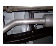
4. Slide muffler #B over headpipe 1.5-2" with the louvers facing towards the converter. Use a jack stand to support the muffler. Use clamp #F to secure the muffler to the headpipe. Do not tighten. Muffler inlet is looking into the louvers.
