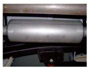
9. Install stainless steel tip. Clamp down. When you have everything in place, firmly tighten all bolts and clamps down securely. Use stainless steel cleaner and a Scotch Brite pad weekly to prevent tip from discoloration. Inspect all fasteners after 25-50 miles of operation and re-tighten as necessary.
