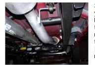
3. Install headpipe #A onto your existing stock front headpipe using stock hardware to secure pipes together. Do not tighten. Use a jack stand to support the converter. Insert welded hangers into rubber grommets.
