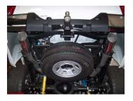
8. Install exit pipes #E. Use clamps #H to secure tailpipes. Do not tighten. May need to trim the exit pipes to best fit your vehicle.
