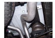
5. Slide the over axle tailpipe #C into the muffler 1.5-2". Use clamp #E to secure tailpipe to muffler. Do not tighten. Insert welded hangers into rubber arommets.
