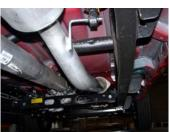
3. Install headpipe #A onto your existing stock front headpipe using stock hardware to secure pipes together. Do not tighten. Insert welded
