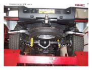
8. Install exit pipes #E. Use clamps #H to secure tailpipes. Do not tighten. May need to trim exit pipes to best fit your vehicle.
