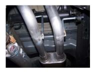
7. Using clamps #G secure both tailpipes to the outlets of the muffler. Rotate tailpipes to best fit your truck.
