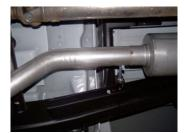
4. Slide muffler #B over headpipe 1.5-2" with the louvers facing towards the converter. Use a jack stand to support the muffler. Use clamp #F to secure the muffler to the headpipe. Do not tighten. Muffler inlet is looking into the louvers.
