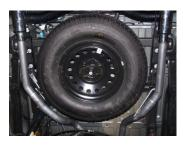
7. Install passenger side tailpipe #C into muffler at least 1.5" to 2". Use clamp #G to secure pipe to muffler. Do not tighten. The tailpipes will both lean towards the driver side for clearance. Insert welded hangers into rubber grommets.
