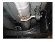
Next, install the headpipe #A. Insert welded hanger into rubber grommet. Use Factory clamp to secure together. DO NOT TIGHTEN.
