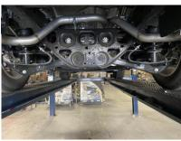
Install the Over Axle Assy. #C into the muffler at least 1-1/2" to 2". #C needs to be installed from the back of the car where the Spare Tire Sits. Use clamp #H to secure pipe to the muffler. Do not tighten. Insert hangers into rubber grommet.
