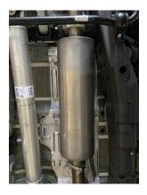
Install muffler onto head pipe #A 1-1/2" to 2" with the louvers facing towards the converter. Use a jack stand to support the muffler. Use clamp #H to the secure the muffler to the head pipe. Do not tighten
