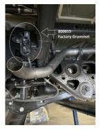
Install metal hangers **#K** using Bolt Kit **#J**. We will Re-use the middle support hanger grommet from the stock exhaust for this bracket.
