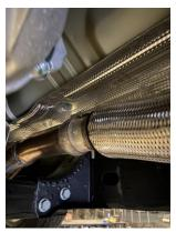
TO REMOVE YOUR STOCK EXHAUST, Un Bolt the back half from the flange LOCATED above the rear suspension, then loosen the front clamp and remove the remaining exhaust. Your Spare Tire & Heat Shield will need to be removed for installation. (FACTORY RUBBER HANGER GROMMETS WILL BE RE-USED, USE WD-40 TO AID IN REMOVAL.)
