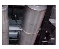
INSTALL MUFFLER #B ONTO HEADPIPE #A 1-1/2" TO 2". USE CLAMP #H TO SECURE THE MUFFLER TO THE HEADPIPE. DO NOT TIGHTEN. SLIDE BAND CLAMP #I ONTO THE MUFFLER AND INSERT THE WELDED HANGER INTO THE RUBBER GROMMET. ATTACH WITH BOLT KIT # K.
