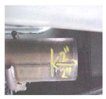
AFTER REMOVAL OF STOCK EXHAUST, CUT 2" OFF YOUR STOCK HEADPIPE.
