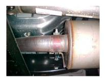
TO REMOVE STOCK **EXHAUST REMOVE IT** FROM THE CLAMP LOCATED IN FRONT OF YOUR STOCK MUFFLER. NOW CUT OFF YOUR STOCK TAILPIPE JUST BEHIND THE MUFFLER AND REMOVE.LEAVE ALL **RUBBER GROMMETS** ON THE HANGER, USE WD-40 TO AID IN **REMOVAL OF EXHAUST AND** HANGERS.
