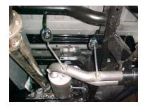
**INSTALL MUFFLER** ASSEMBLY #A ONTO STOCK PIPE 1-1/2" TO 2". SLIDE WELDED HANGERS INTO RUBBER **GROMMETS YOU** MAY NEED TO ADJUST WELDED HANGERS TO FIT INTO YOUR GROMMETS, USE A JACKSTAND TO SUPPORT YOUR MUFFLER. USE CLAMP #B TO SECURE IT TO YOUR HEADPIPE. DO NOT TICHTEN
