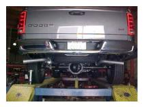
INSTALL EXIT PIPES #E, USE CLAMPS #G TO SECURE TO THE TAILPIPES.
