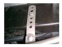
MEASURE 19 <sup>1</sup>/<sub>2</sub>" FROM THE REAR OF THE FRAME AND USE THIS HOLE AND BOLT ON HANGER #H. USE THE 2<sup>ND</sup> HOLE FROM THE TOP.
