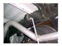
INSTALL MUFFLER #B ONTO HEADPIPE 1-1/2" TO 2". USE CLAMP #I TO SECURE THE MUFFLER TO THE HEADPIPE. DO NOT TIGHTEN. SLIDE BAND CLAMP #J ONTO THE MUFFLER AND INSERT THE WELDED HANGER INTO THE RUBBER GROMMET. ATTACH WITH BOLT KIT #K.
