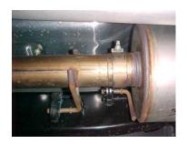
YOU MAY NEED TO HEAT IT UP FOR EASIER REMOVAL. LEAVE ALL RUBBER GROMMETS IN PLACE. USE WD-40 TO AID IN REMOVAL OF EXHAUST AND HANGERS.
