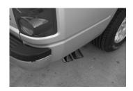
Install the stainless tips. Clamp down. To clean your stainless tips use any stainless cleaner. Now go back and tighten all clamps, nuts and bolts. Start from the front and work back.
