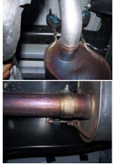
1. To remove the stock exhaust un-clamp the tailpipe just after the stock muffler. Then un-clamp the stock muffler. Leave all rubber grommets in place. Use WD-40 to aid in removal of exhaust.
