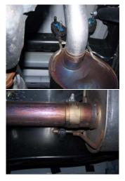
1. To remove the stock exhaust remove it from in front of the stock muffler. Disengage the welded hangers using WD-40 from the OEM rubber grommets. Do not damage or remove the rubber grommets as you will re-use them to mount your new system. Now, cut off tailpipe and remove exhaust.
