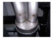
**6.** Install driver side tailpipe #D 1½-2" into muffler and use clamp #G to secure to muffler. Attach clamp #G to hold up to the hanger #H. DO NOT TIGHTEN.
