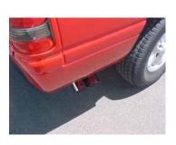
INSTALL THE STAINLESS TIPS. NOW GO BACK AND START AT THE FRONT AND TIGHTEN ALL CLAMPS AND HANGERS.
