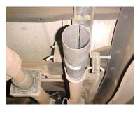
INSTALL HEADPIPE # A AND ATTACH TO THE STOCK EXTENSION PIPE USING CLAMP #F
