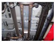
2. Remove the stock exhaust at the 2-bolt flange located in front of the muffler. Disengage the welded hangers from the OEM rubber grommets. Use WD-40 to help in the process. Do not damage or remove the rubber grommets as you will reuse them to mount your new system. Now, unbolt the tailpipe and remove exhaust. Do not throw away stock flange bolts, as you will reuse them.
