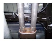
5. Install extension pipe #D into muffler. Use clamp #J to secure. Do not tighten. Next install driver side extension pipe #E into muffler using clamp #J to secure. Do not tighten. Insert welded hanger into rubber grommet.
