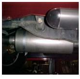
INSTALL MUFFLER # C ONTO YOUR RESONATOR 1 ½" –2". USE CLAMP # G TO SECURE MUFFLER TO THE PIPE, DO NOT TIGHTEN.
