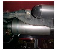
INSTALL MUFFLER # C ONTO YOUR RESONATOR 1 ½" –2". USE CLAMP # G TO SECURE MUFFLER TO THE PIPE, DO NOT TIGHTEN.
