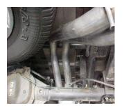
INSTALL PASS. SIDE TAILPIPE # E INTO MUFFLER 1 ½"-2". USE CLAMP # H TO SECURE PIPE TO MUFFLER, DO NOT TIGHTEN.
