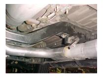
INSTALL Y-PIPE # A & M ONTO STOCK FLANGES USE YOUR STOCK HARDWARE TO SECURE INSERT WELDED HANGER INTO RUBBER GROMMET, DO NOT TIGHTEN.
