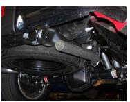
INSTALL EXIT PIPES # E ONTO TAILPIPES. ROTATE OUT TO THE SIDES; ATTACH TO TAILPIPES WITH CLAMPS # H.
