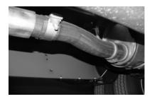
TO REMOVE YOUR STOCK EXHAUST, UNBOLT AND REMOVE THE CLAMP LOCATED JUST IN FRONT OF THE MUFFLER. FOR EASIER REMOVAL OF THE FACTORY EXHAUST, CUT OFF THE STOCK TAILPIPE JUST BEHIND THE MUFFLER AND REMOVE. LEAVE ALL RUBBER GROMMETS ON THE HANGERS. USE WD-40 TO AID IN REMOVAL OF EXHAUST AND HANGERS.
