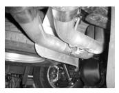
INSTALL DRIVER SIDE OVER AXLE TAILPIPE # D INTO MUFFLER 1½ TO 2". INSERT WELDED HANGER INTO RUBBER GROMMET, USE CLAMP # G TO SECURE PIPE TO MUFFLER. THIS PIPE WILL GO INTO THE DRIVERS SIDE OUTLET. DO NOT TIGHTEN
