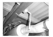
TO REMOVE YOUR STOCK EXHAUST, UNBOLT AND REMOVE THE CLAMP LOCATED JUST IN FRONT OF THE MUFFLER. FOR EASIER REMOVAL OF THE FACTORY EXHAUST, CUT OFF THE STOCK TAILPIPE JUST BEHIND THE MUFFLER AND REMOVE. LEAVE ALL RUBBER GROMMETS ON THE HANGERS. USE WD-40 TO AID IN REMOVAL OF EXHAUST AND HANGERS.
