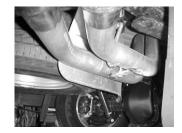
INSTALL PASSENGER SIDE OVER AXLE TAILPIPE # C INTO MUFFLER 1½ TO 2". INSERT WELDED HANGER INTO RUBBER GROMMET, USE CLAMP # G TO SECURE PIPE TO MUFFLER. THIS PIPE WILL GO INTO THE PASSENGER SIDE OUTLET. DO NOT TIGHTEN
