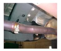
TO REMOVE YOUR STOCK EXHAUST, REMOVE IT FROM THE CLAMP LOCATED JUST IN FRONT OF THE MUFFLER REMOVE HANGERS FROM RUBBER GROMMETS BY PULLING EXHAUST TOWARDS THE REAR OF THE VEHICLE, USE WD-40 TO AID IN REMOVAL, LEAVE GROMMETS IN PLACE.
