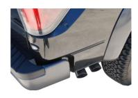
Install stainless steel tips. Clamp down. When you have everything in place, firmly tighten all bolts and clamps down securely. Use stainless steel cleaner and a Scotch Brite pad weekly to prevent tip from discoloration.
