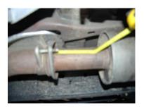
TO REMOVE YOUR STOCK EXHAUST, MEASURE 6" FROM THE 2-BOLT FLANGE LOCATED IN FRONT OF YOUR STOCK MUFFLER AND CUT.
