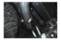
INSTALL PASS. SIDE TAILPIPE # C INTO MUFFLER 1  $\frac{1}{2}$ " TO 2". INSERT HANGER INTO RUBBER GROMMET, USE CLAMP # G TO SECURE PIPE TO MUFFLER. DO NOT TIGHTEN.
