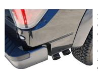
Install stainless steel tips. Clamp down. When you have everything in place, firmly tighten all bolts and clamps down securely. Use stainless steel cleaner and a Scotch Brite pad weekly to prevent tip from discoloration.
