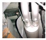
INSTALL DRIVERS SIDE TAILPIPE # D INTO MUFFLER 1 ½" TO 2". INSERT HANGERS INTO RUBBER GROMMETS, USE CLAMP # G TO SECURE PIPE TO MUFFLER. DO NOT TIGHTEN. THE TAB ON THIS PIPE SHOULD GO ON BOTTOM OF PASSENGER SIDE PIPE USE BOLT KIT # H TO SECURE TOGETHER.
