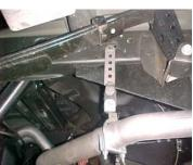
ON DRIVER SIDE MEASURE 17-1/2" FROM THE REAR OF THE FRAME FORWARD. USE HANGER # I. USE THE TOP HOLE OF THIS HANGER. USE HARDWARE PROVIDED. REPEAT FOR PASS. SIDE.
