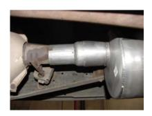
SLIDE INLET OF MUFFLER ASSEMBLY #A ONTO CATALYTIC CONVERTER. USE CLAMP #B TO SECURE. DO NOT TIGHTEN.
