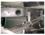
ON DRIVER SIDE: ATTACH REAR TAILPIPE HANGER #I TO FRAME BY REMOVING THE 18MM HITCH BOLT. THEN RE INSTALL BOLT WITH HANGER (IF YOU DO NOT HAVE A FACTORY HITCH USE BOLT KIT #K TO ATTACH HANGER #I & #J TO THE FRAME RAIL.
