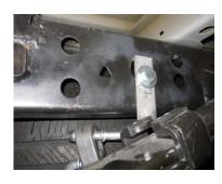
ON DRIVER SIDE: ATTACH REAR TAILPIPE HANGER #I TO FRAME USING BOLT KIT PROVIDED
