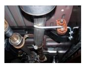
INSTALL HEADPIPE # A INTO STOCK FLANGE ATTACH WITH BOLT KIT PROVIDED. DO NOT TIGHTEN. INSERT WELDED HANGER INTO RUBBER GROMMET.
