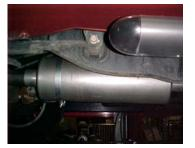
LAY OUT THE GIBSON EXHAUST ON THE FLOOR AND COMPARE PART #'S TO THE DRAWING. TO **REMOVE YOUR FACTORY** EXHAUST UN-BOLT YOUR TAILPIPE AT THE 2-BOLT FLANGE LOCATED BEHIND YOUR STOCK MUFFLER USE WD-40 TO AID YOU IN REMOVAL OF HANGERS FROM RUBBER GROMMETS.
