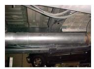
NEXT, INSTALL RESONATOR # B 1 1/2"-2" ONTO Y-PIPE USE CLAMP # I TO SECURE PIPES TOGETHER, DO NOT TIGHTEN.
