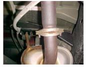
LAY OUT THE GIBSON EXHAUST ON THE FLOOR AND COMPARE PART #'S TO THE DRAWING. TO REMOVE YOUR FACTORY EXHAUST UN-BOLT YOUR TAILPIPE AT THE 2-BOLT FLANGE LOCATED BEHIND YOUR STOCK MUFFLER. USE WD-40 TO AID YOU IN REMOVAL OF HANGERS FROM RUBBER GROMMETS.
