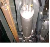
ON DRIVER SIDE: ATTACH REAR TAILPIPE HANGER #I TO FRAME BY REMOVING THE 18MM HITCH BOLT. THEN RE INSTALL BOLT WITH HANGER (IF YOU DO NOT HAVE A FACTORYHITCH USE BOLT KIT #L TO ATTACH HANGER #I TO THE FRAME RAIL. REPEAT ON PASSENGER SIDE.
