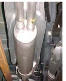
INSTALL MUFFLER # B ONTO HEADPIPE 1 ½" TO 2". USE CLAMP '# G TO SECURE MUFFLER TO HEADPIPE. DO NOT TIGHTEN. USE A JACK STAND TO HOLD UP THE MUFFLER. OUTLETS SHOULD BE LEVEL.
