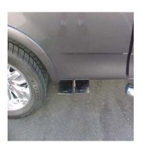
**INSTALL THE** STAINLESS STEEL TIP. **USE ANY ALUMINUM** OR STAINLESS STEEL CLEANER TO POLISH TIP. NOW TIGHTEN ALL CLAMPS AND BOLTS.
