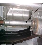
INSTALL NEW HEADPIPE # B AND ATTACH USING CLAMP # E TO FACTORY PIPE.
