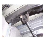
INSTALL WELDED HANGER INTO RUBBER GROMMET
