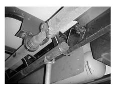
INSTALL HEADPIPE #A ONTO STOCK HEADPIPE AND ATTACH WITH #E. THE FLARED END GOES ONTO THE STOCK HEADPIPE. NEXT INSTALL HANGER #D ONTO HEADPIPE HANGER. INSERT WELDED RODS INTO RUBBER GROMMET. DO NOT TIGHTEN.
