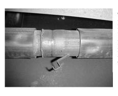
TO REMOVE STOCK EXHAUST, UN-BOLT AT THE FIRST JOINT, APPROXIMATELY 35" IN FRONT OF THE STOCK MUFFLER AND CUT CLAMP OFF.
