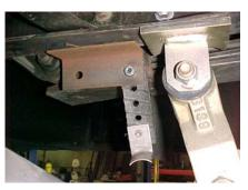
AFTER TAILPIPE #C IS IN PLACE AND HANGER #F IS IN PLACE. INSTALL HANGER #G CLAMP WITH CLAMP #E TO FRAME.
