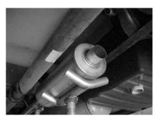
INSTALL MUFFLER #B ONTO HEADPIPE #A WITH INLET FACING TOWARDS HEADPIPE USING HANGER #D TO ATTACH. DO NOT TIGHTEN. MUFFLER INLET IS LOOKING INTO THE LOUVERS.
