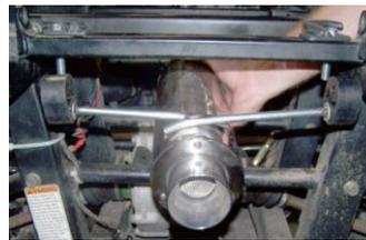
14. After everything is in place, go ahead and tighten up the flange nuts at the head. **Use caution when tightening down the header exhaust nuts.** Do not over tighten as it can cause the factory studs to break. You only need to make a snug fit much like a spark plug install.
