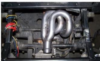
8. Install Gibson hanger and bracket using stock bolts.
