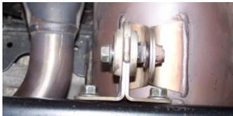
4. Then undo the bolt on the bracket at the center of the stock muffler. Now remove bracket from frame. Save Bolts.
