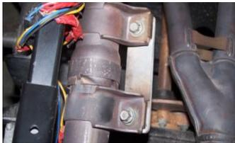
5. Next, unbolt the 2 bolts at the bracket located where the stock header and s-bend are connected. Then slide s-bend off of header.
