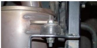
3. To unbolt the stock exhaust, first unbolt the top nut and bolt from the rubber grommet at the front of the muffler.
