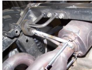
9. Then slide the dome gasket #G over the outlet of the header.
