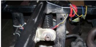
2. To remove the stock exhaust, you must remove the bed. Lift up the bed and disconnect the wiring harness. Then remove it from the 2 pins at the frame. Remove the cotter pins, and then take out frame pins. Now remove the bed.
