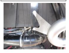
5. Bolt the tailpipe brackets to the rear under bed bracket. You will use Bolt Kit # B. Use the large fender washers on the back side of the top hole. You may have to loosen the factory bracket to adjust for fitment. Do not tighten until all bolts are installed. Install both sides.
