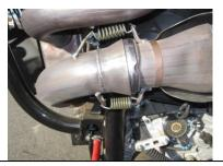
4. Next install the Gibson Muffler assembly. Install the top hanger mounts first then slide the inlet over the factory head pipe re using the factory gasket and springs. Once in position, install Headpipe and top muffler springs.
